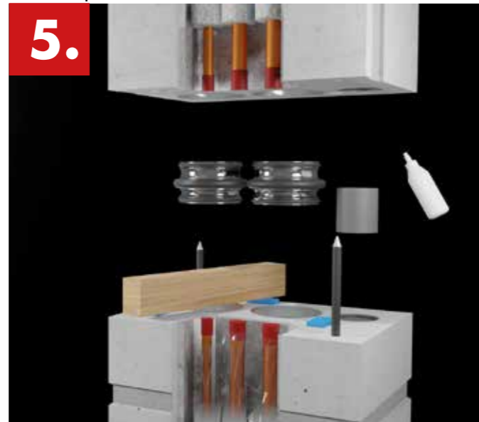
5. Carefully lubricate the pipe ends and connectors with lubricant. Install the lubricated connectors on the surface of the upper unit. Use a safety block.
